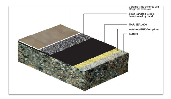
Immediately before the application of any component of the system, the substrate shall be dry, with any remaining dust or loose particles removed using clean, dry, oil-free compressed air, industrial vacuum, cloth-wipe or a combination.
